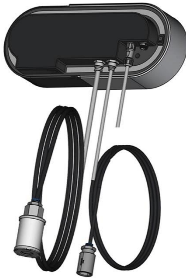
Fig. 23: Sensor with hose lines
