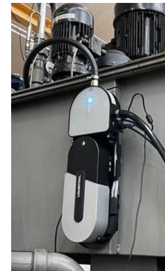
Vertical on machine (Emulsion inlet at top)
