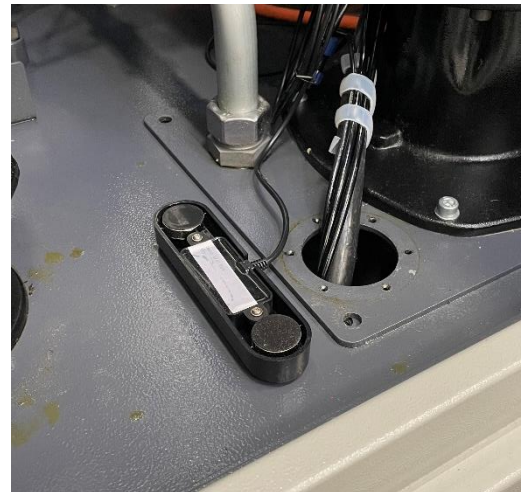
Opening for ultrasonic sensor too small
