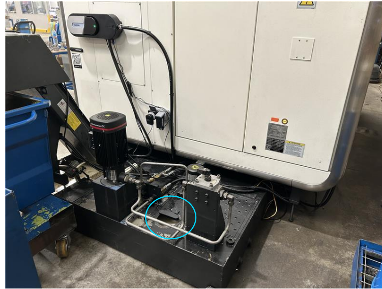
Opening for ultrasonic sensor too small
