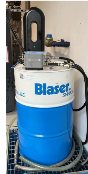
Opening for ultrasonic sensor too small
